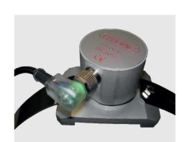
活塞式蓄壓器超音波量測活塞位置 Piston position measured with ultrasound sensor
